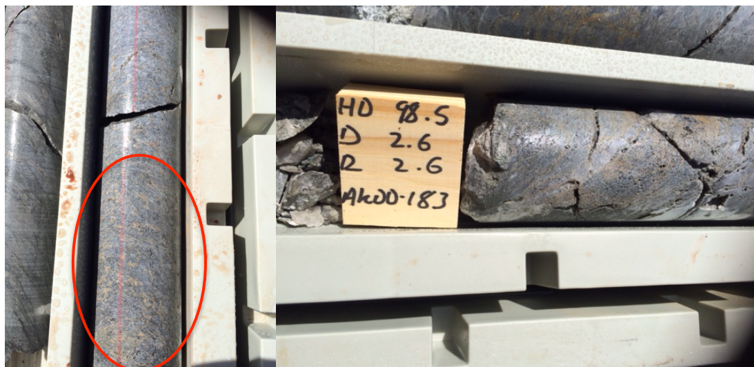
Figure 2 – Honey-brown sphalerite (zinc) and silver sulphosalts intersected by AKDD183 at 95.5 m (left) and 98.6 m (right)
