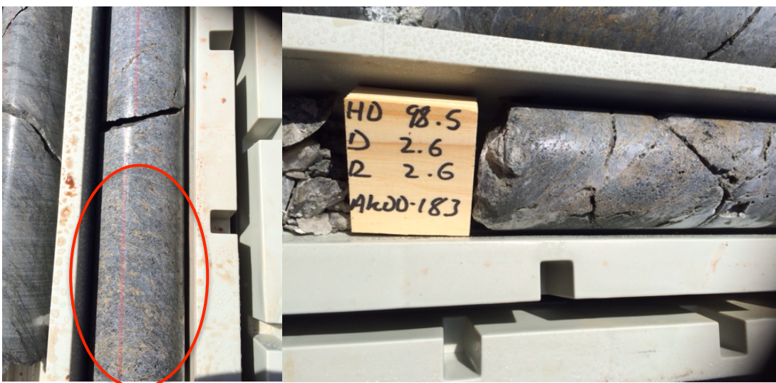
Figure 3 – Honey-brown sphalerite (zinc) and silver sulphosalts intersected by AKDD183 at 95.5 m (left) and 98.6 m (right)
