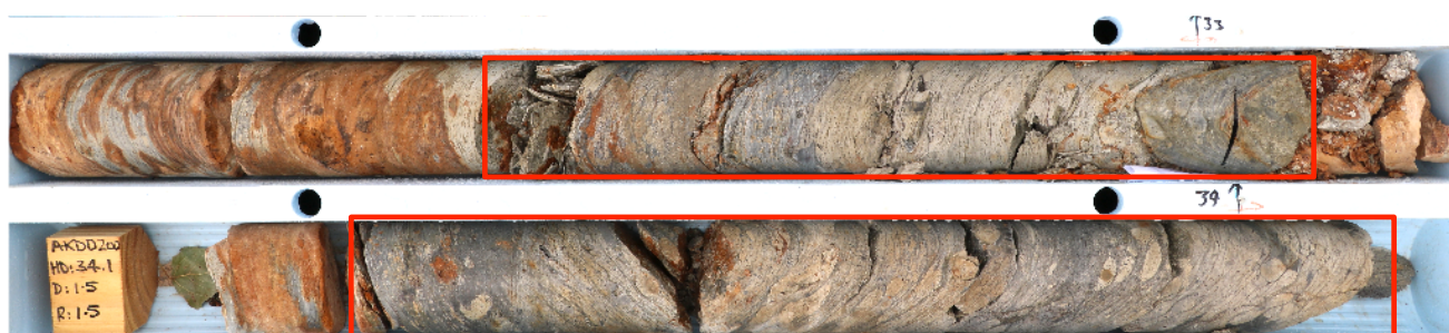
Figure 4 – Photo of AKDD200 drill core including a highlighted section of the mineralised interval: 1.0 m @ 2.2% Pb, 8.3% Zn (10.5% Pb+Zn), 250 g/t Ag and 0.2 g/t Au from 213.4 m.
