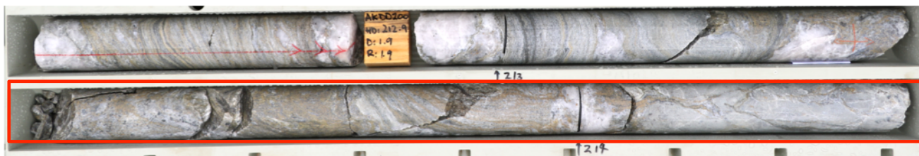
Figure 4 – Photo of AKDD200 drill core including a highlighted section of the mineralised interval: 1.0 m @ 2.2% Pb, 8.3% Zn (10.5% Pb+Zn), 250 g/t Ag and 0.2 g/t Au from 213.4 m.
