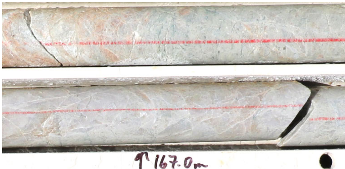
Figure 9 – AWT004 at 167.0m: 30 cm core lengths – Fine crystalline quartz- and feldspar-phyrlic tonalite with strong pervasive illite-chlorite-k feldspar alteration and intense silicification.
