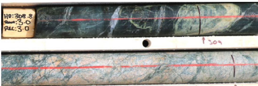
Figure 7 – AWT003 at 308.8 and 309.8 metres: 30 cm core lengths - Strong selective and fracture controlled chlorite-magnetite-epidote altered mafic tuff with stockwork quartz-calcite-epidote-pyrite-pyrrhotite veins and small (1 metre wide) potassic altered quartz- feldspar-phyric quartz-monzonite with stockwork quartz-actinolite-epidote-chlorite-pyrite veins.
