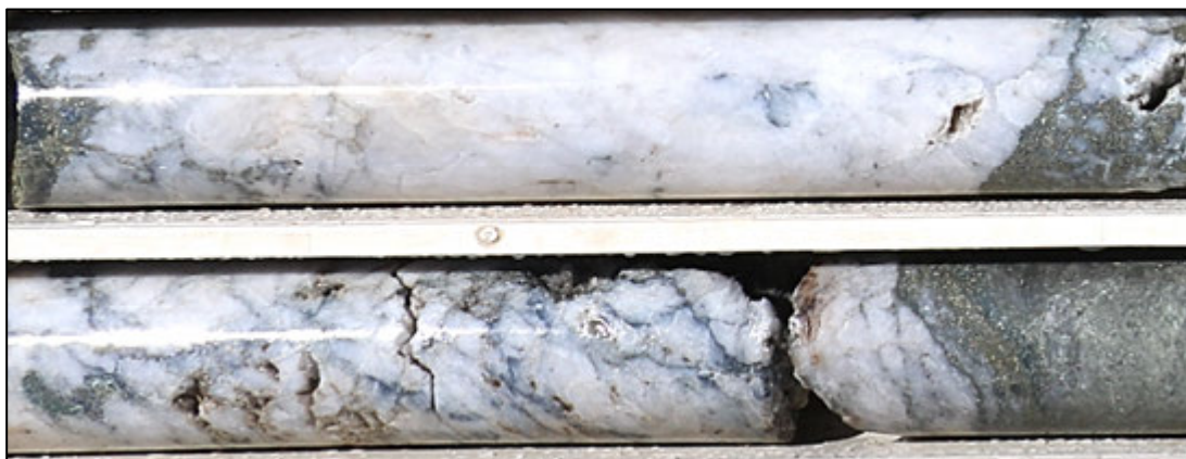
Figure 3 - AWT002 drill core at 211.5 metres (top row) and 212.5 metres (bottom row). Stringer molybdenite in massive quartz vein with intense sericite altered and pyritic wallrock. Host unit is a clay altered, chlorite-actinolite greywacke.
