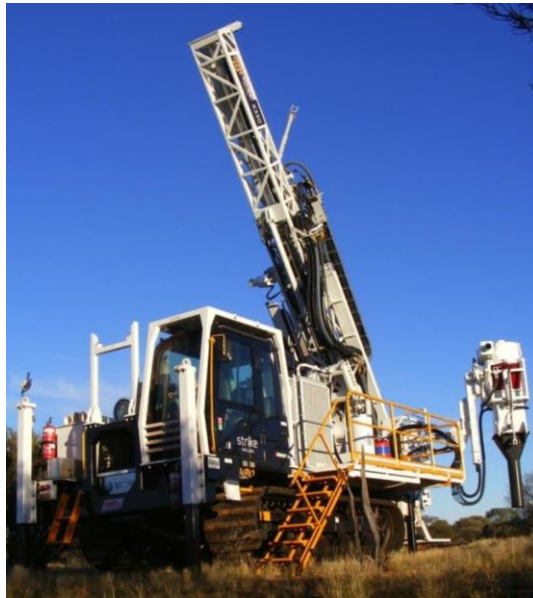
Figure 2: Strike Drilling X350 AC/RC Drill Rig
