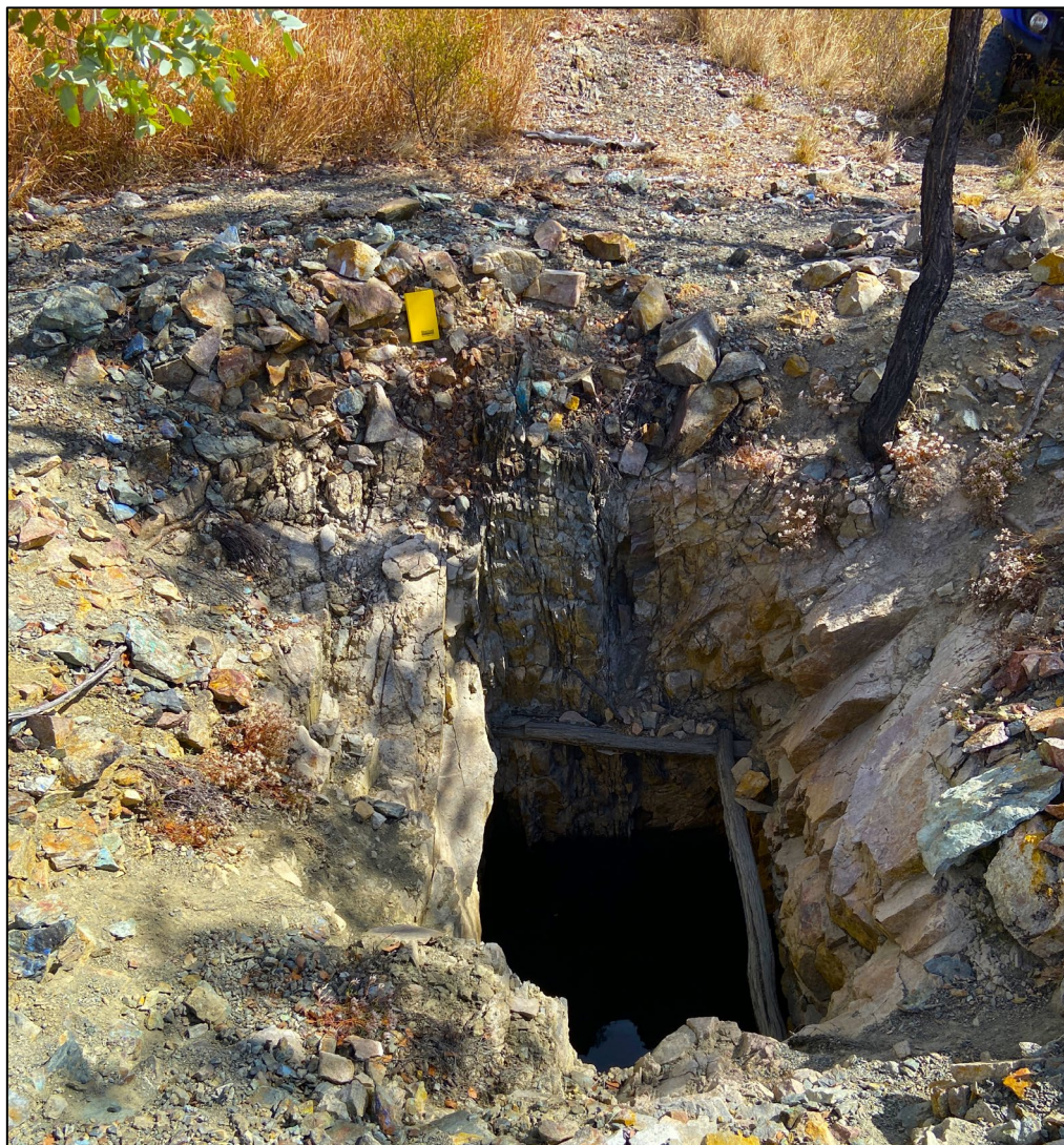
Figure 2. Visible copper mineralisation at Copper Dyke (azurite and malachite) hosted within siliceous vein. Inset shows a hand specimen of copper mineralisation (malachite) hosted in siliceous veining.
