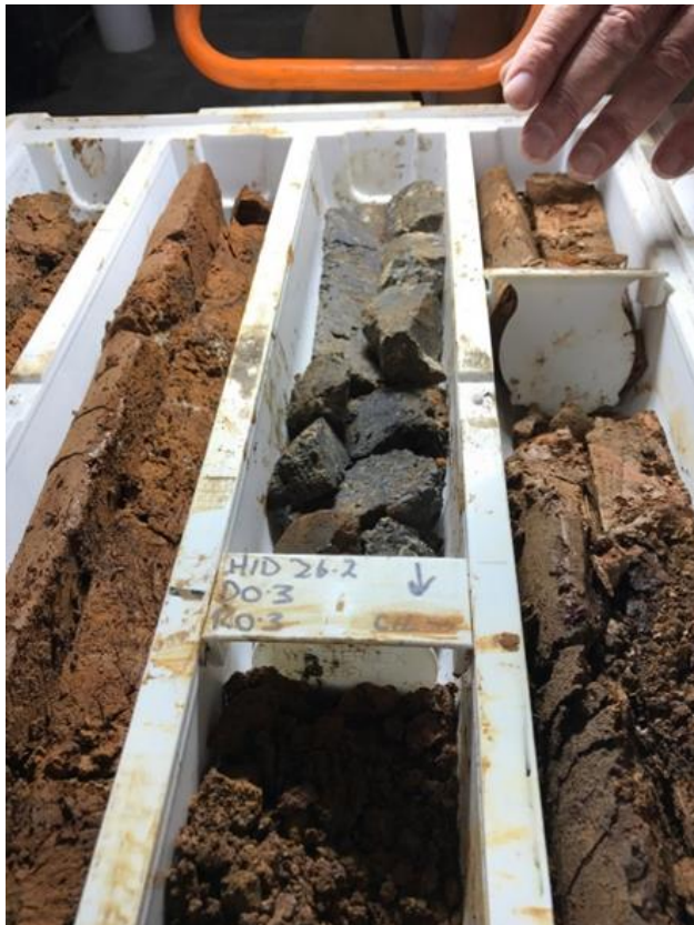
Figure 6 – High grade cobalt-nickel mineralisation from around 26.0 m depth in drill hole AGSD0004. As a rule of thumb, higher cobalt and nickel grades correspond to darker material in the drill core. The core in the centre of the left image contains strong mineralisation measuring 0.69 % cobalt and 2.07 % nickel.
