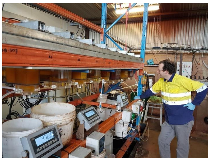
Figure 1 – Scandium solvent extraction test work underway yesterday at Simulus Engineers in Perth.
