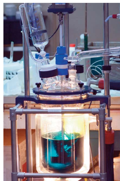
Crystal production, pink-red solution is cobalt sulphate, blue-green is nickel sulphate
