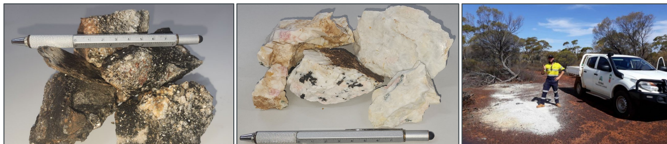
Figure 12: Left and Centre images - Pegmatite samples 600m southeast of AHID0024 showing mica zone. Assays awaited. Right hand image - Drill hole 01MNRC0115 with 0-30m (EOH) of LCT prospective white intermediate-felsic porphyry.
