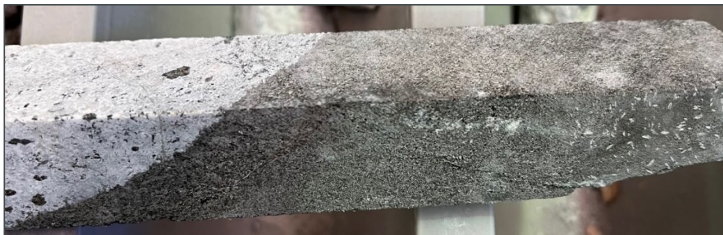
Figure 10: AHID0024: Section of core from 0.85m @ 0.34\% \text{Li}_2\text{O} , 3,392ppm Cs, 4,222ppm Rb, 51ppm TI from 368.75m with the Li-Cs-Rb-Tl anomalism within the dark biotite-rich interval on contact with the plagioclase-biotite porphyry.
