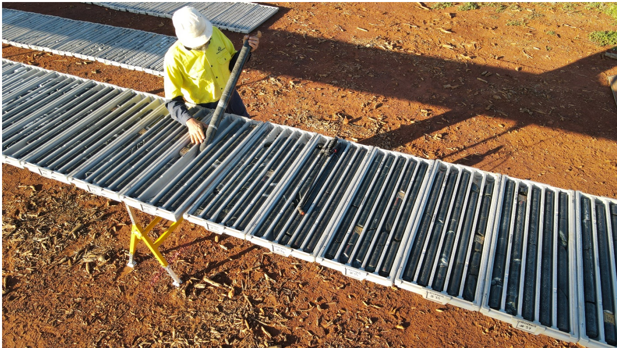
Figure 7. Logging of NIC ultramafic and mafic rocks in NDD0005
