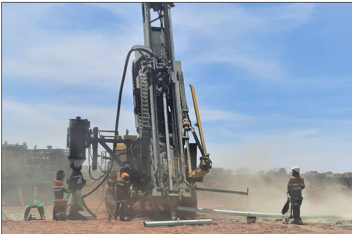
Figure 1. RC rig operating at Niobe.
