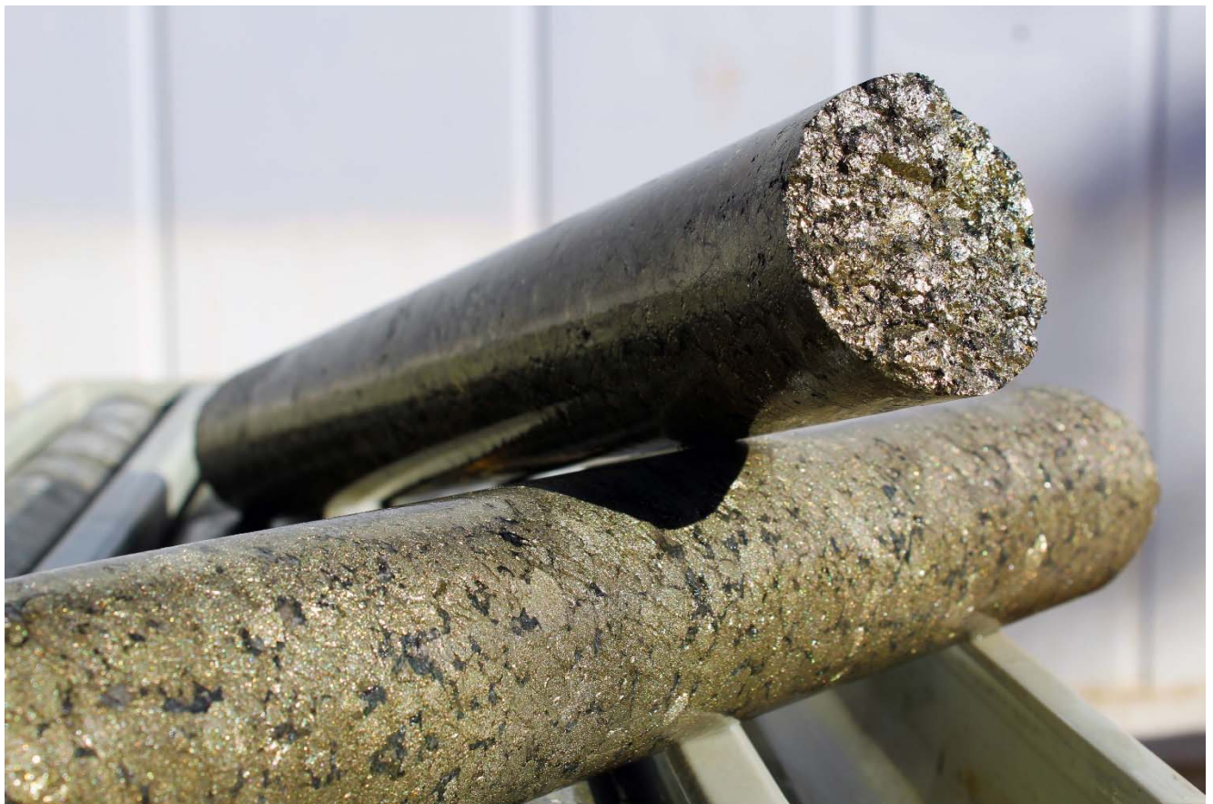
Figure 1. Massive cobaltiferous pyrite mineralisation intersected by diamond drilling at Railway deposit, Thackaringa Project
