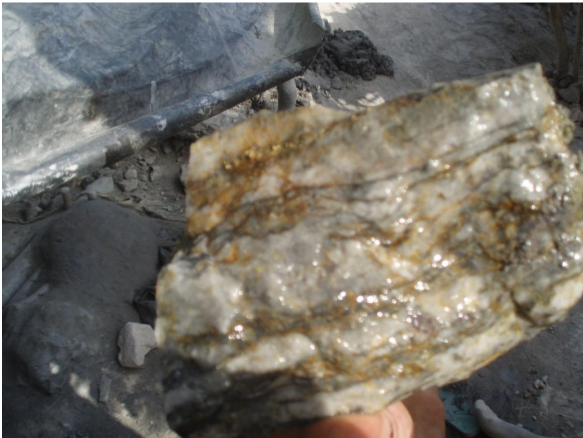
Photograph 2. Sample of "ribbon textured" quartz veining with a 5 mm band of visible gold (top left) from the Linnguekoto Prospect.
