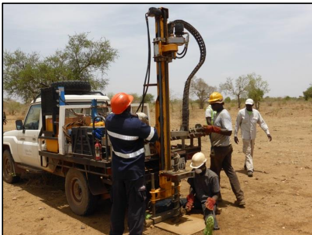
Photographs 1 & 2. Golden Rim's auger rig, and the lateritic profile of a typical auger hole.
