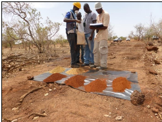
Photographs 1 & 2. Golden Rim's auger rig, and the lateritic profile of a typical auger hole.
