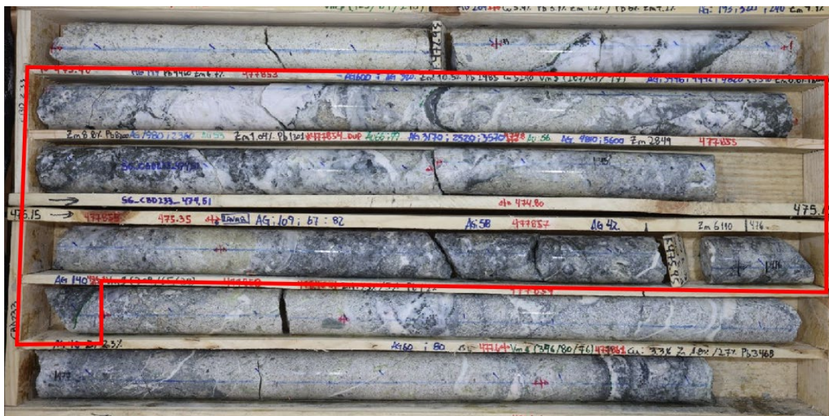
Figure 5. CBD233 Main lode mineralised quartz breccia, 2.7m @ 507g/t AgEq from 473.4m to 476.1m.
