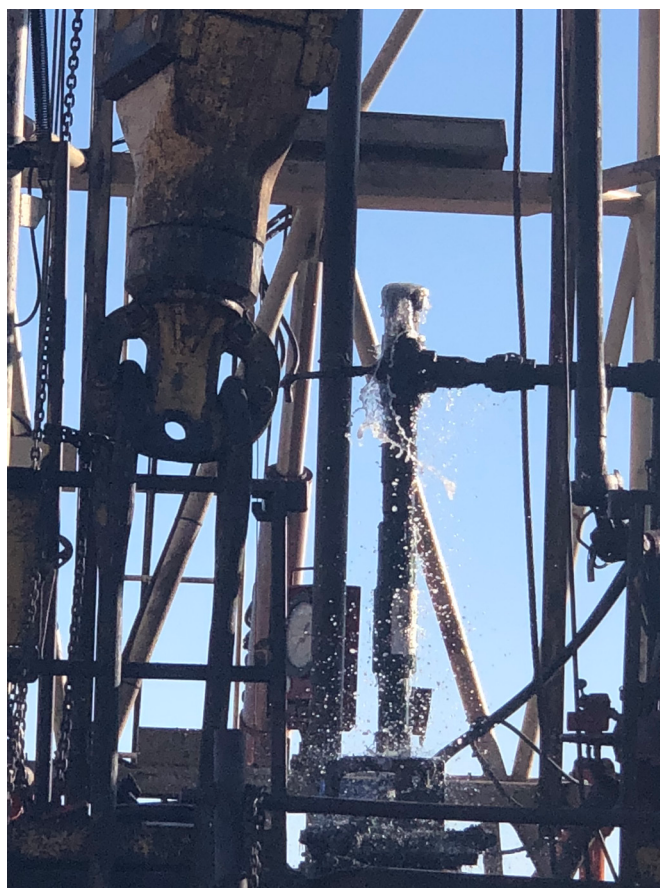
Figure 2: shows the supersaturated brine free flowing from the tubing of the workover rig.
