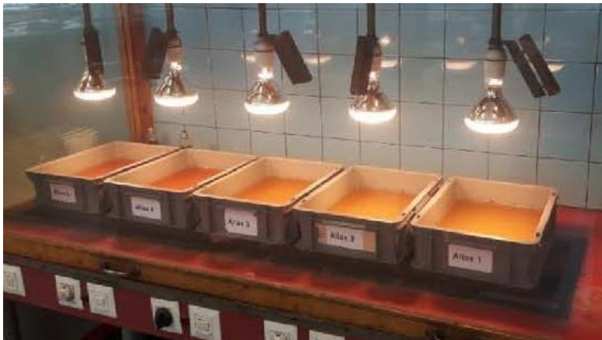
Figure 1: Photographs of the brine during evaporation by heat lamps.
