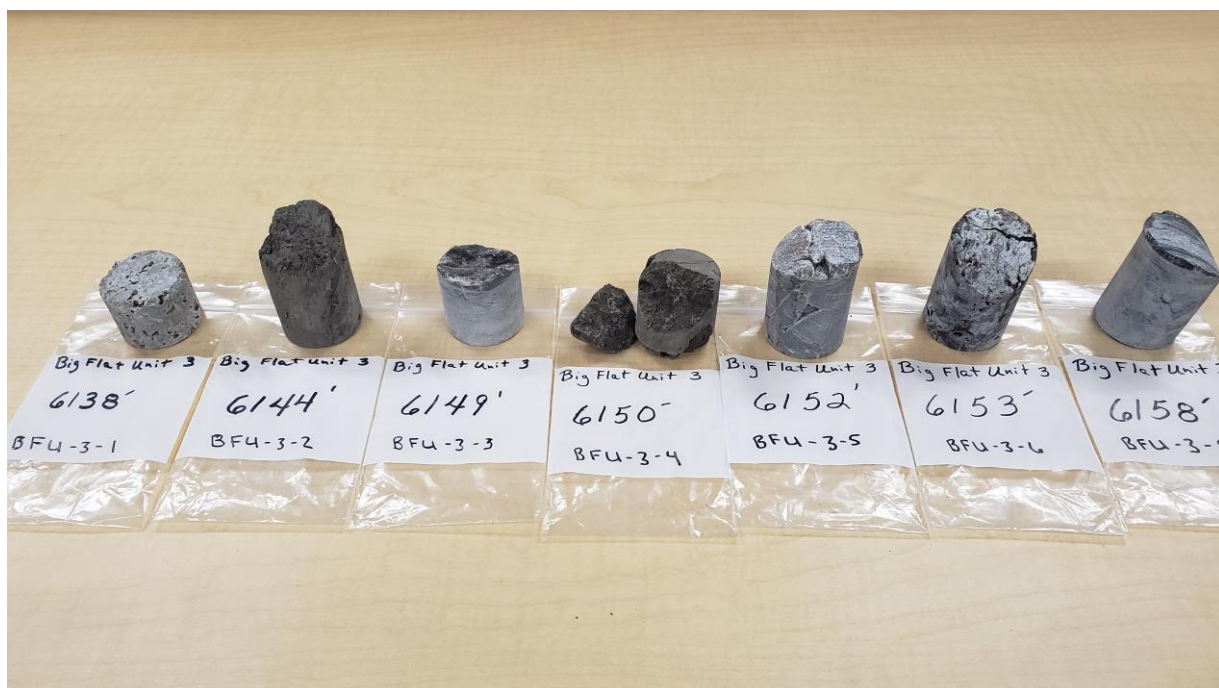
Figure 1: Photos of Diamond Core Plugs from Clastic 31
