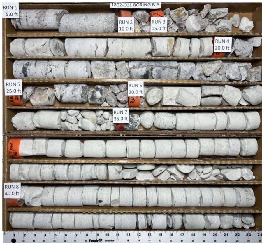
Figure 3: The core from borehole 5 (B-5)
