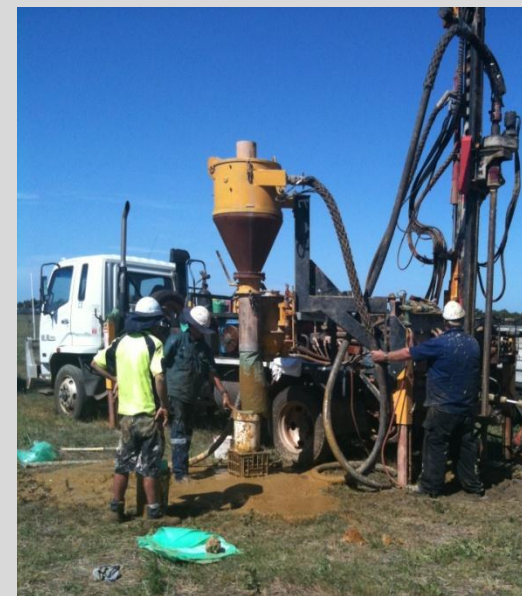
First phase RC drilling at Southdown Extension iron ore project, Western Australia
