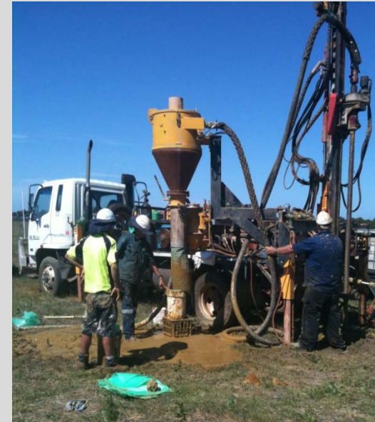
First phase RC drilling at Southdown Extension iron ore project, Western Australia
