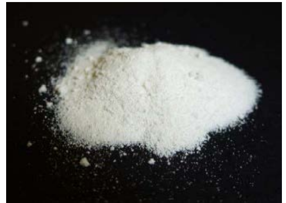
Figure 1. Photo of final alumina sample using AMMG's processing technology
