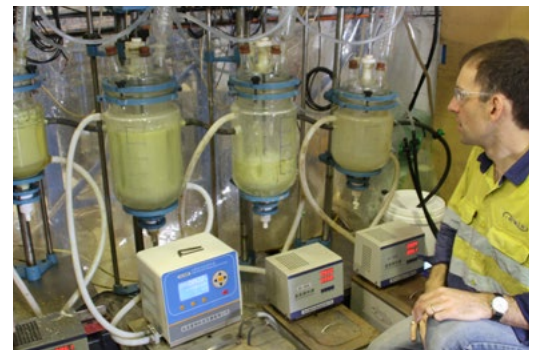
Fig 1. Optimisation test work (continuous leaching test work) is underway on the process flowsheet developed by AMMG
