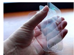
Fig 4. Artificial sapphires used in touch-screen displays and smartphone components
