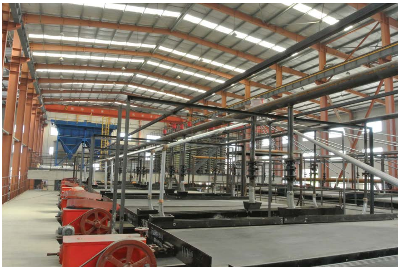
Shaking tables, Astron's Yingkou mineral separation plant, China and storage bins below.
