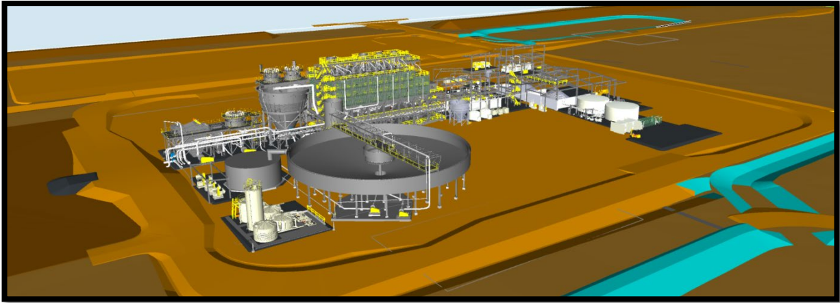
Figure 18 – Thickener and process water ponds
