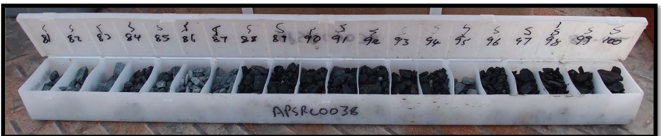
Photo 2: Chip tray from hole APSRC0038 depth 80-100m showing sulphides in a basaltic unit in each one metre interval. Note the colour changes from leucocratic depths 81-83, 86-87 and 95 to melanocratic phases and the 1% sulphide content at 98m.
