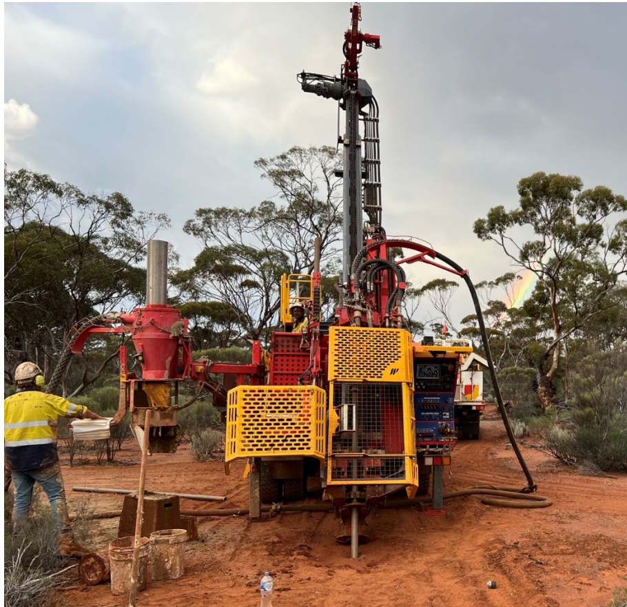
Figure 1: Aircore drilling completed at Ryans Find.
