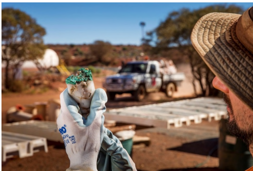
Diamond core from the target zone in hole FGDD002 at the Forrest copper-gold discovery
