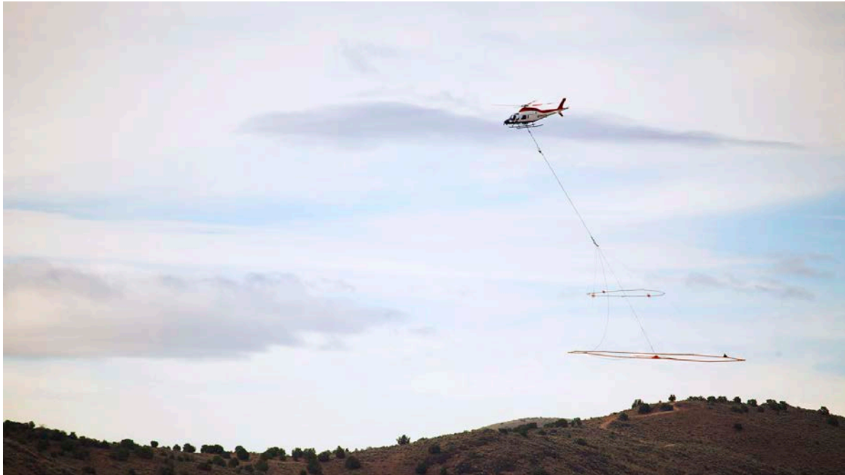
Figure 1: Helicopter-borne Versatile Time-Domain Electromagnetic (VTEM™ Max) geophysical system
