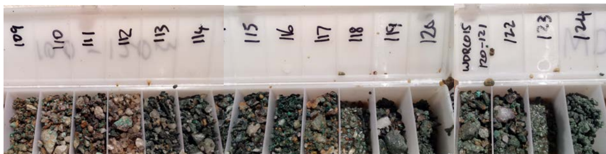
Figure 9 – Sieved chip samples from WDR015, 108-124m. Malachite mineralisation associated with quartz veining and foliated Narracoota Formation. Metre displayed is “Depth To” for metre sample. Base of Complete Oxidation at 112 metres.
