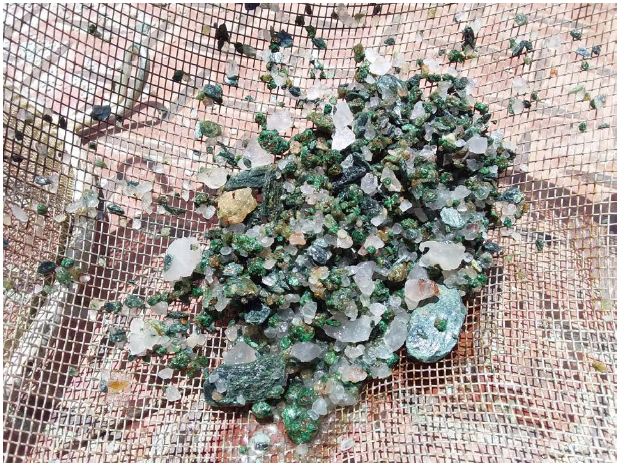
Figure 5 – Sieved chip sample from FPRC029, 298-299m. Abundant malachite mineralisation associated with quartz veining and foliated Narracoota Formation. Assay result – 3.62% Cu and 0.42g/t Au. Mesh size of sieve is 2mm.
