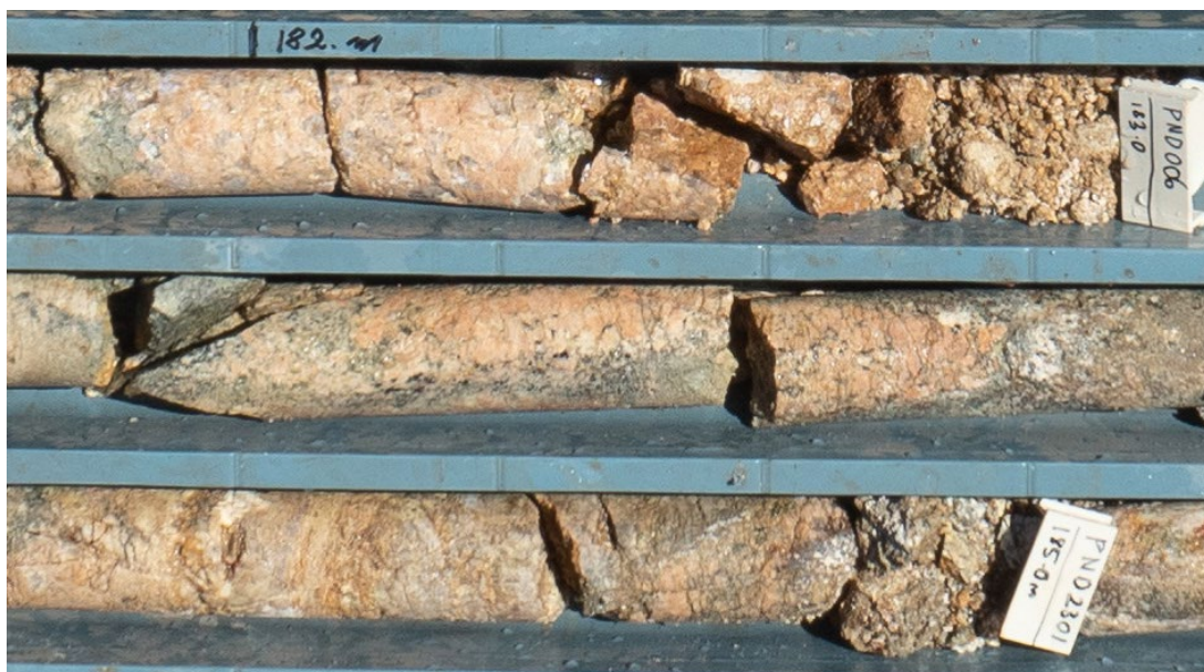
Figure 2 – PND006 Drill Core: Weathered pegmatite with weakly anomalous Ag, As, Bi (section shown covers part of interval 182.7 to 185.1m)
