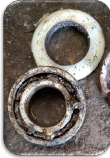
Removed bearing showing damage
