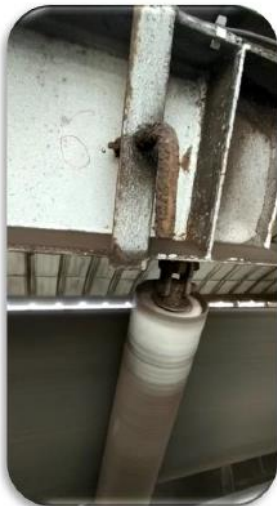
Photo of roller in operation. Noise not exceptionally unusual. No issue detected by Adani
