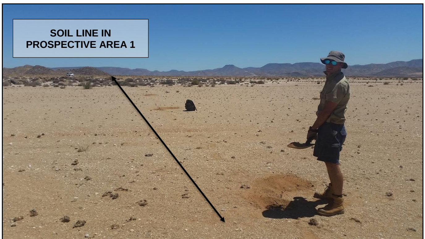
Plate 2: View looking SSW along new soil line in P1, designed to define pegmatite under shallow cover
