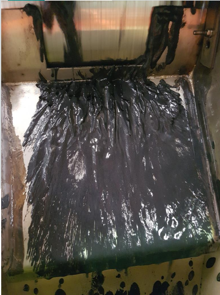
Gabanintha Vanadium Concentrate on Low Intensity Magnetic Separation Unit
