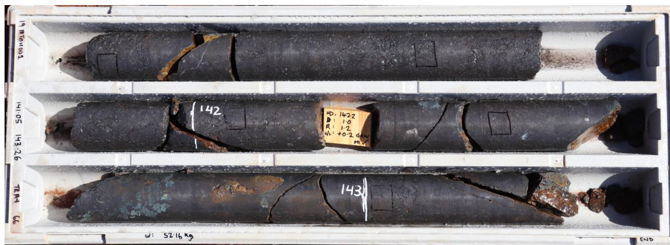
Plate 2 - Fresh Massive Magnetite in Diamond drill core from 19MTDH001 on site at the Gabanintha Project
