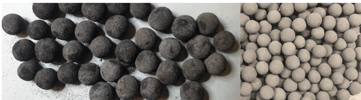
Figure 4 - Vanadium Rich Iron Concentrate Pellets Produced During Bench-Scale Roast Testing
