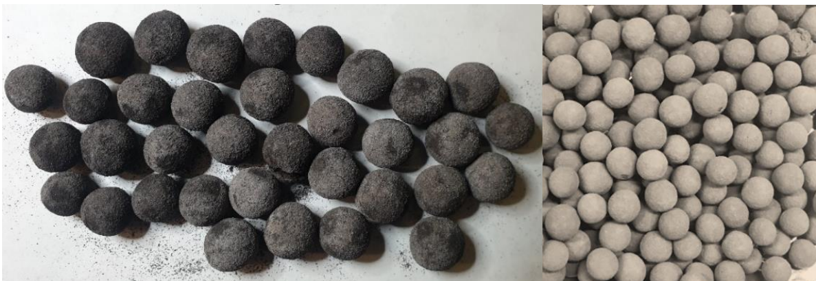
Figure 4 - Vanadium Rich Iron Concentrate Pellets Produced During Bench-scale Roast Testing
