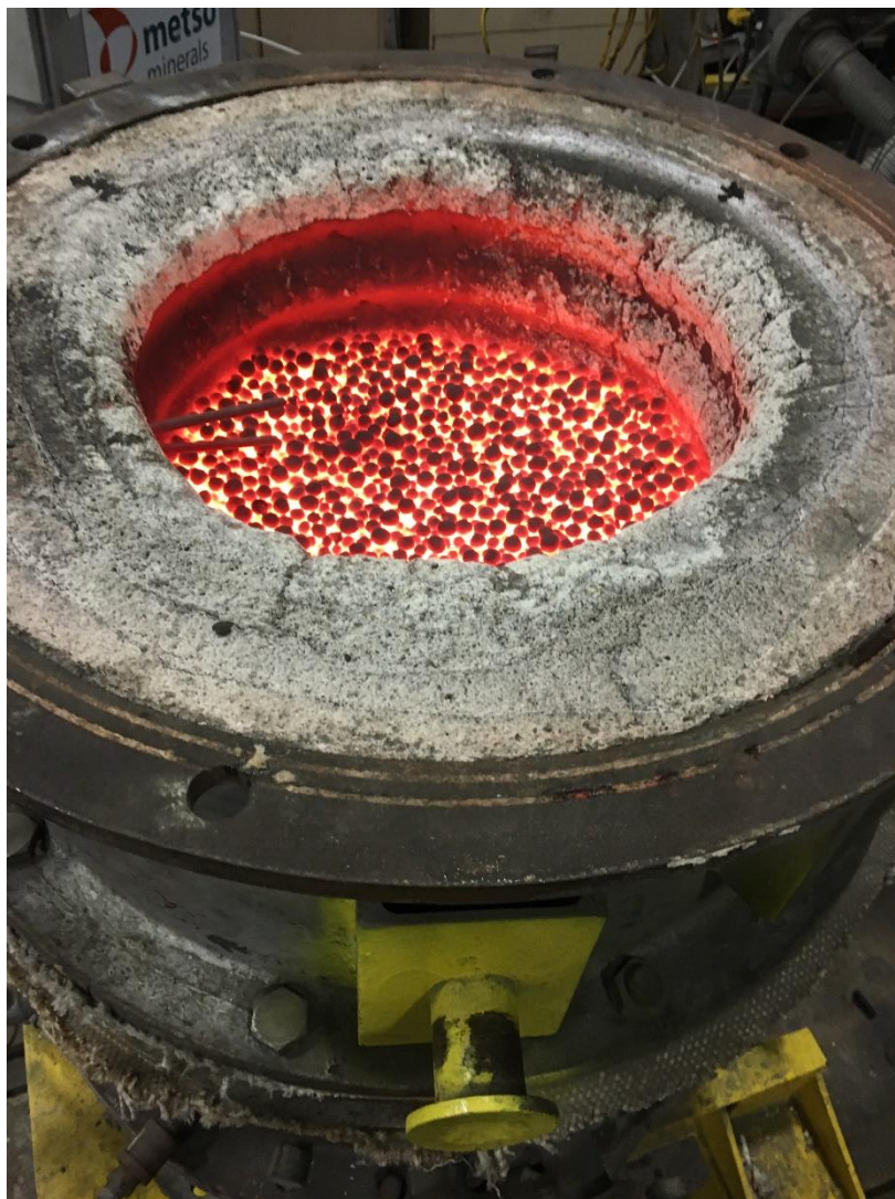
Figure 9 - Grate Kiln Pellet Testwork at Metso
