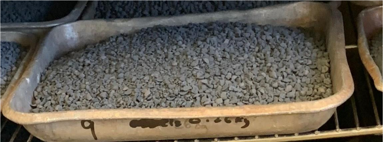
Figure 2: Pilot feed - roasted pellets crushed to <6.3mm
