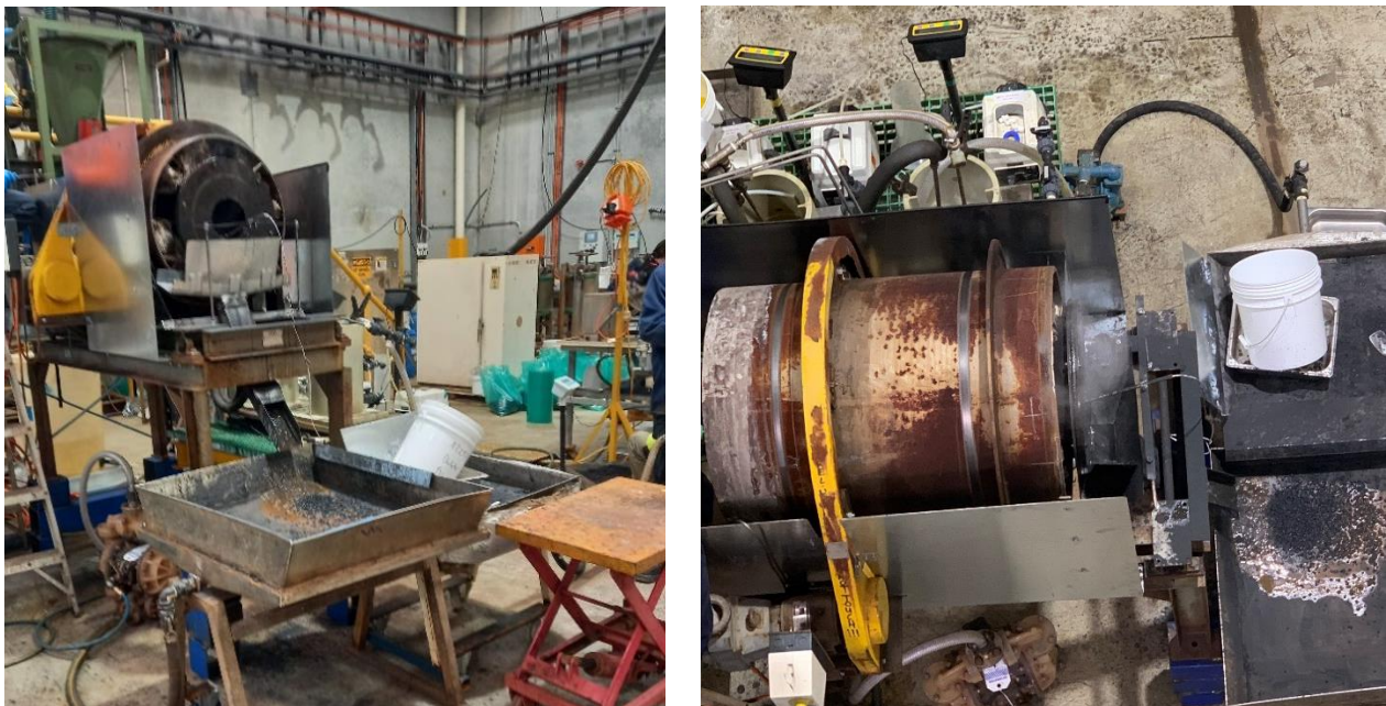
Figure 1. Pilot set-up showing rotating drum and filtering operations
