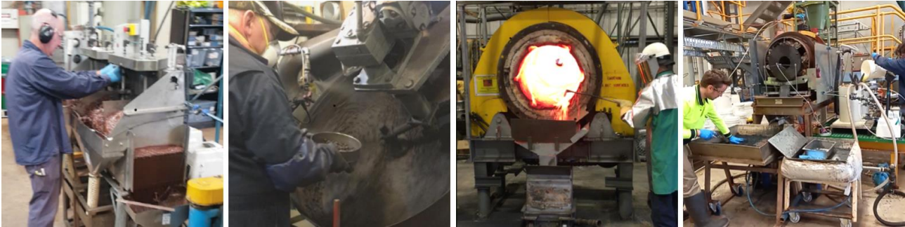
Figure 4 - AVL's process includes reverse flotation, pelletisation, salt-roasting and leaching; demonstrated at full pilot-scale from left-right
