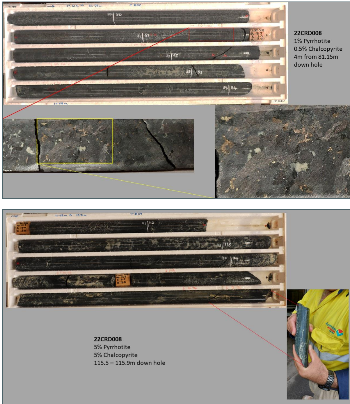
Figure 4: Core photos of Pyroxenite unit and Chalcopyrite veinlet. Top – 22CRD008 at 81.15m Bottom 22CRD008 at 115.5m
