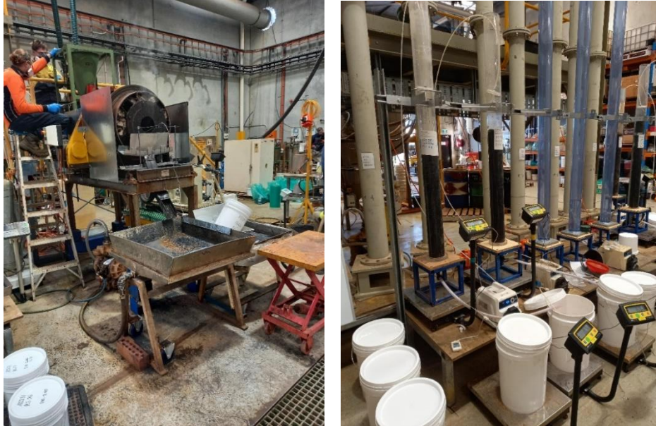
Figure 3 - Pilot scale leach process utilising a primary drum leach followed by a column leach
