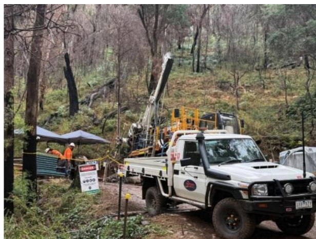
Figure 3. Photograph of the diamond rig on site at the Happy Valleys deposit, set up to complete deep hole AMD023.
