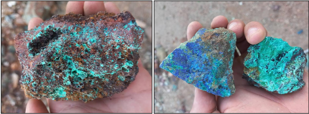
Figure 2: Gossanous sample that returned 10.32% Cu and 4.68g/t Au (left). Malachite and azurite mineralisation (right).
