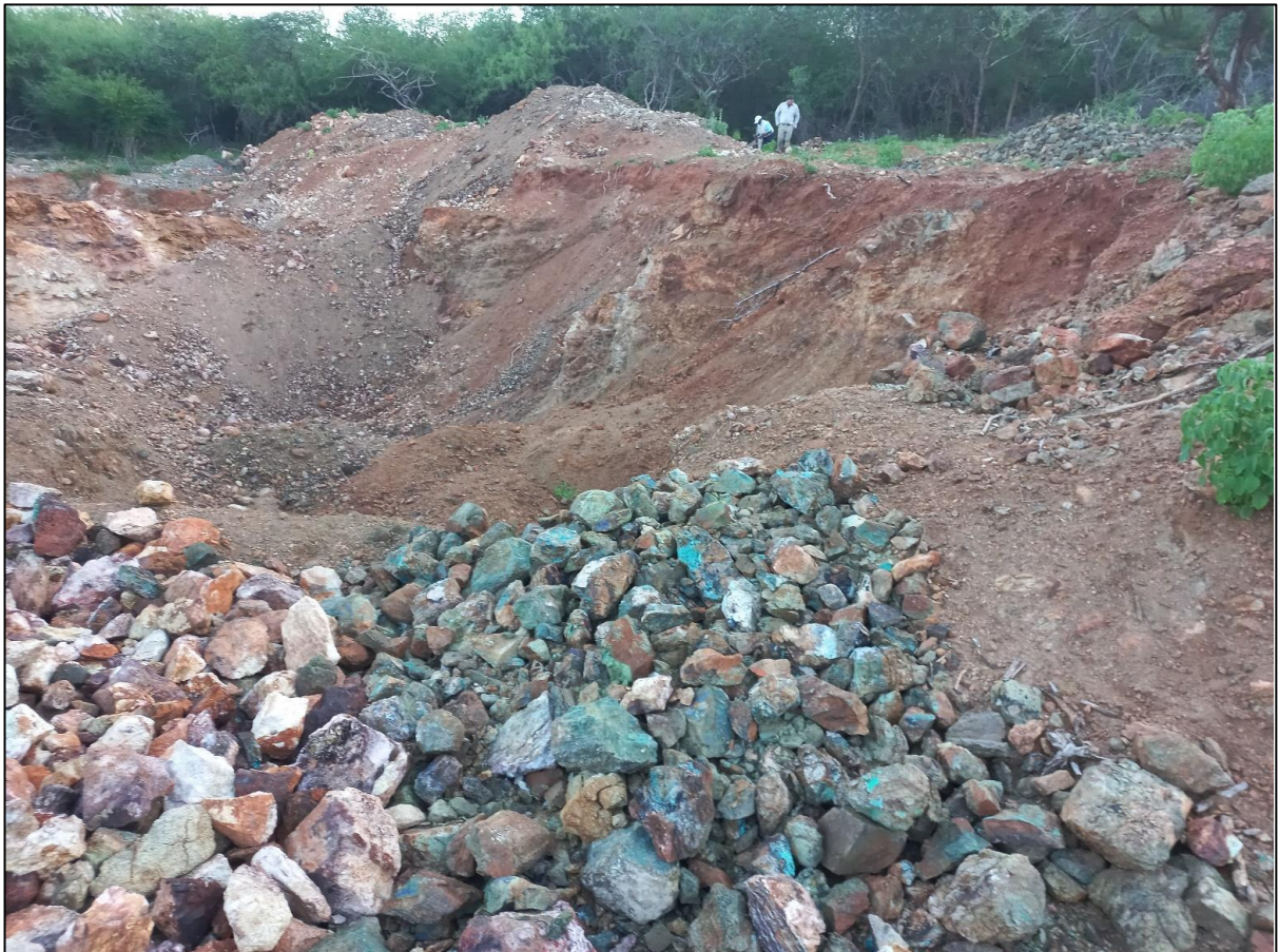
Figure 3: Excavated pit with small stockpile of copper-rich ore.
