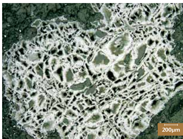
Figure 1: Polished section (PS), (x50). Gossanous/goethite box-work with a fine trellis texture interpreted to represent original chalcopyrite now completely oxidised and leached.
