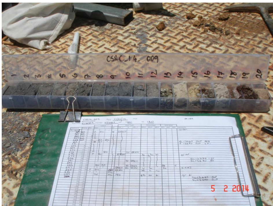
Plate 7. RC chips from CSRC14_009 after logging (note graphite from surface).
