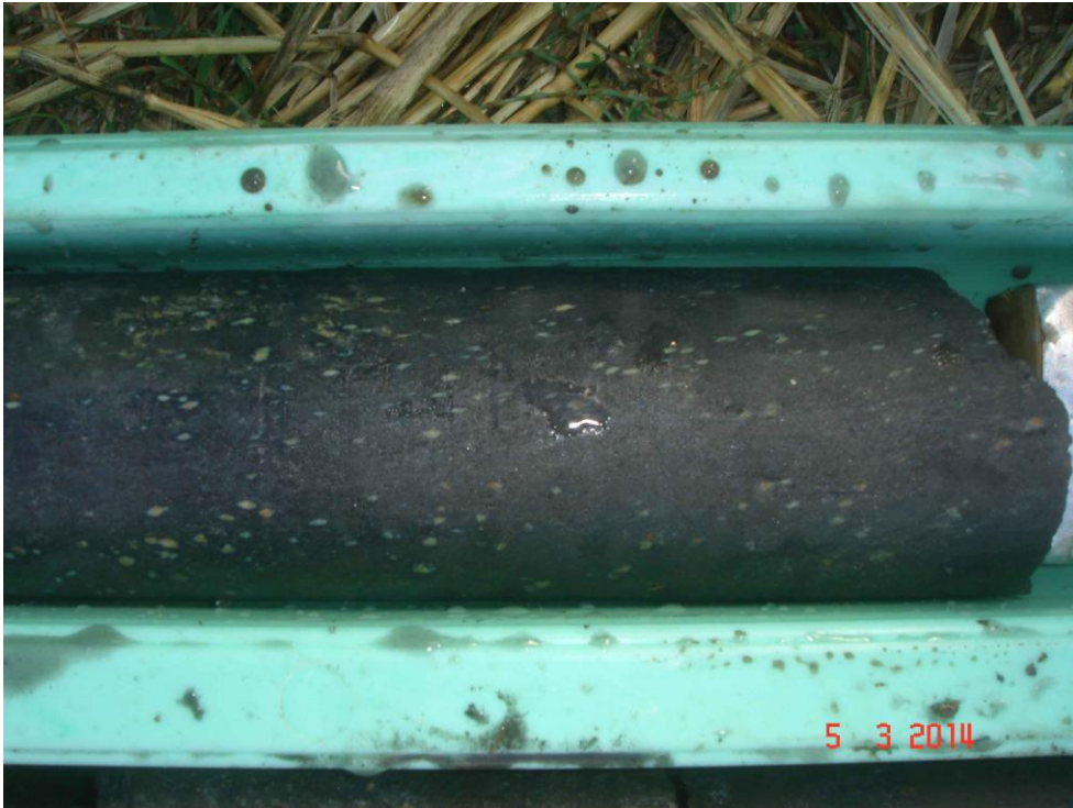
Plate 6. CSDD14_001 4.1m down hole graphite ore
