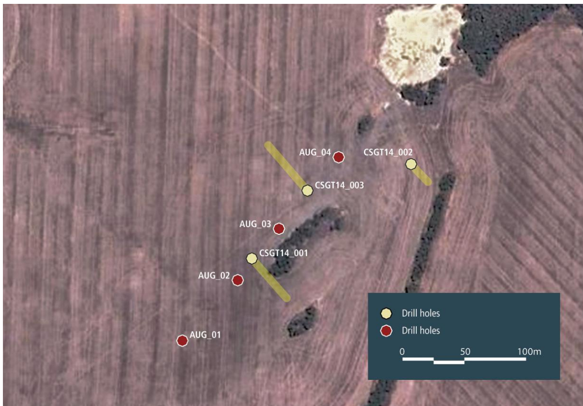
Plate 1. Location of Auger and diamond holes drilled at Campoona Shaft in 2014 (lines denote hole directions).
