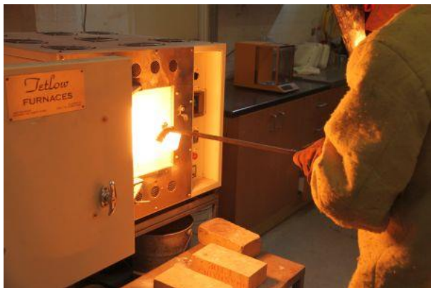
Figure 2: Removing crucibles from the furnace
