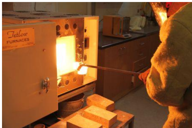
Removing deadburn magnesia from furnace
