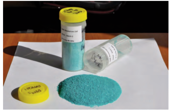
Photo above: High purity (+99.98%) Nickel sulphate products produced from the continuous pilot plant.
